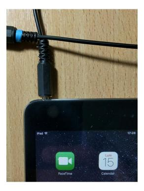
If you have a protective case for your device make sure the case thickness does not interfere with the complete insertion of the 3.5mm jack.
